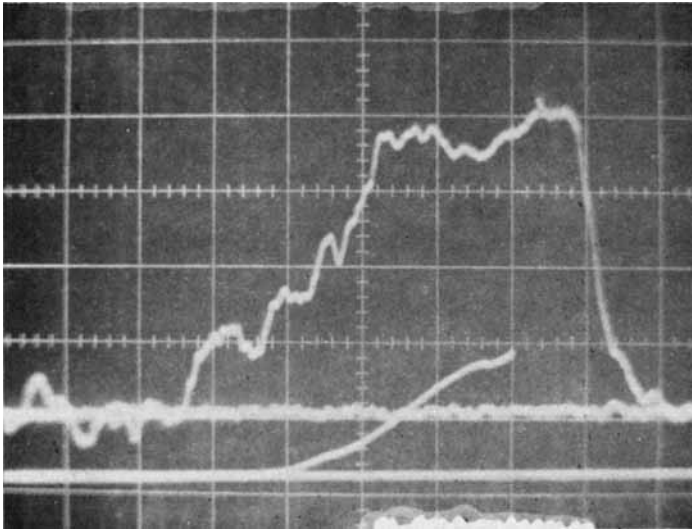
Fig. 3. Typical oscilloscope record for 1000-S-O aluminum alloy.
